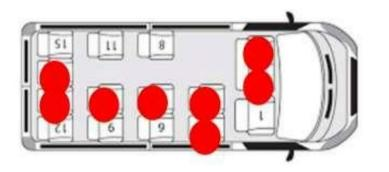
Example of a bus with reduced numbers of passengers - the seats coloured red should be left empty
